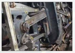
The extensive network of lubrication pipes that feed the axle boxes, motion parts and cylinders have been replaced, and this has included some painstaking work in ensuring that the final pipe work arrangements mirror the original BR design drawings.
